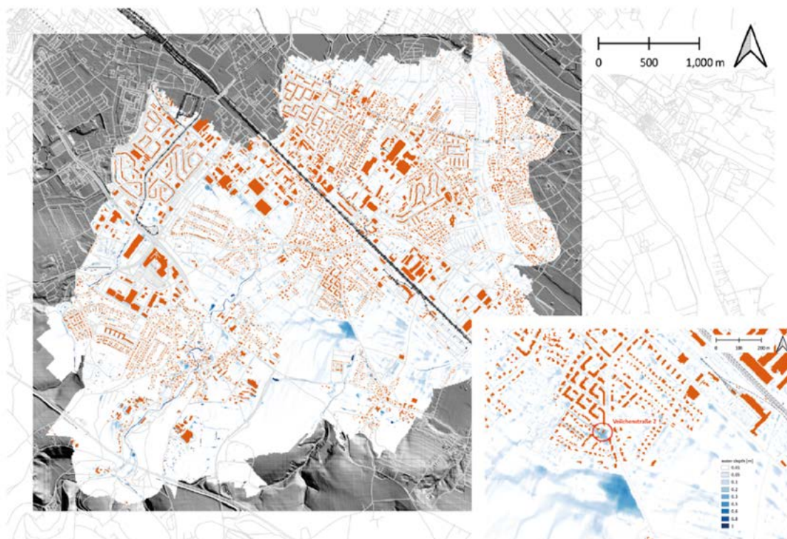
Figure 1: Simulated maximum surface inundation for the heavy precipitation event of 27th May, 2014 in the Lockwitzbach area of Dresden. The inset shows a plausibility check, comparing a reported basement inundation of a building (red circle) with the simulated inundation.
