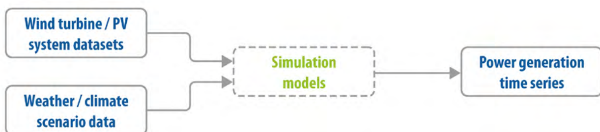
Figure 1. Flowchart of the numerical simulations showing the involved data and the information flow.
